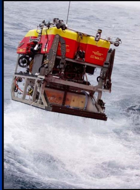
Step 3: Left: When Isis is underneath the gantry, the pilot turns parallel to the ship, and the winch lifts the vehicle out of the water. Good judgment is needed in rough seas to avoid the cable going slack, then snatching, as waves go by. Step 4: Right: Nearly home - Isis then latches firmly into the head of the gantry, to avoid swinging as it is brought on deck.
