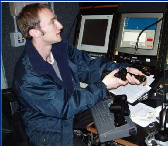
The manipulators are operated from the control container, using the 'Mini Masters'
