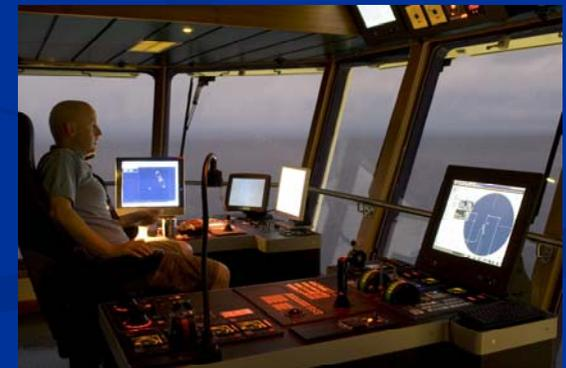
A bridge officer at the DP station, in constant communication with the ROV navigator
