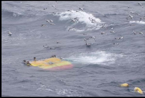
Step 1: Vehicle surfaces, staying away from the side of the ship, stern to, while the buoyancy floats are removed one-by-one.
