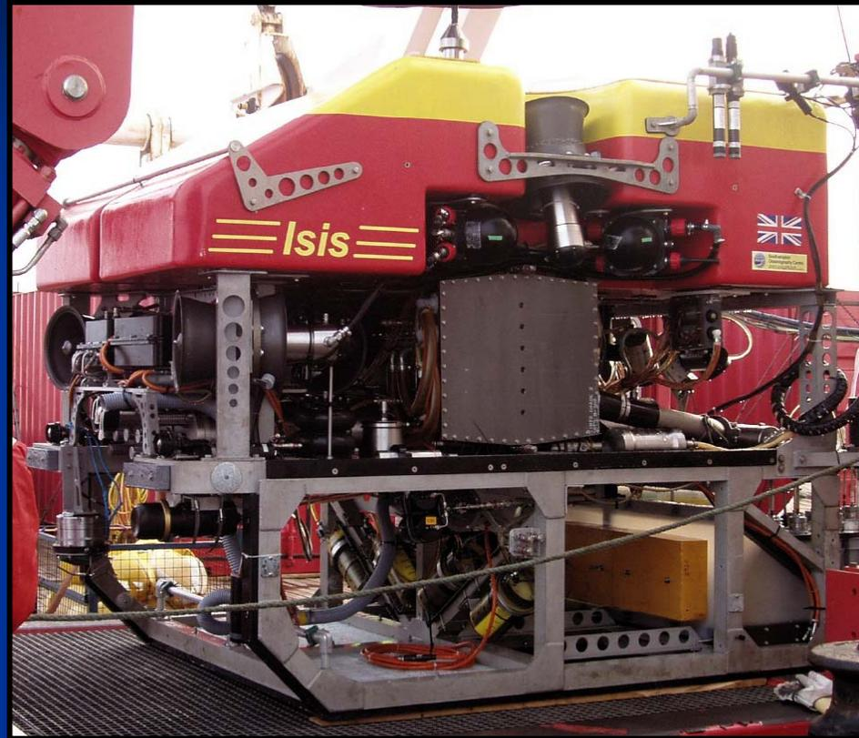
*Framework made from welded hollow section and structural aluminium. Corrosion protected with anodes and ground-fault detectors. Most electronics housed in titanium pressure vessels.*
