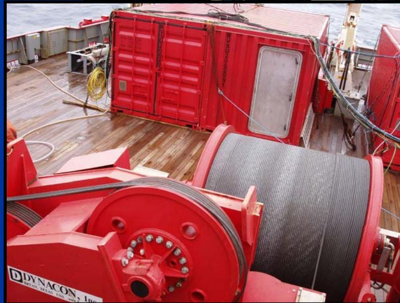
Winch and cable drum with 10km cable. Three optical fibres for data and three conductors at 3kV for power.
