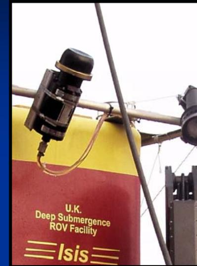
The MS1000 echosounder is a pencil beam 875kHz single beam device that scans mechanically to generate an image
